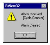
Reading the status register automatically clears the alarm flags. Once an alarm is enabled, it can be armed for the next event by writing a higher value into the alarm register or resetting the counter.
